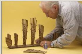
Stan starts his assembly Up-Side-Down! Measure spacing between bents and glue. Use a 90° framing square to check accuracy.
