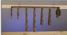
The bridge is literally 'hanging' at this stage, supported by the temporary support beam.
